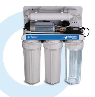
This compact RO system is ideal for residential drinking water purification. The 5-stage system is designed with a 5-micron sediment prefilter, a second stage GAC carbon filter, followed by our patented 2-in-1 BLOCKFREE filter, designed for optimal RO membrane protection.
