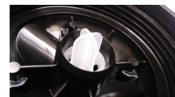
Removable filter cartridge centering plug
